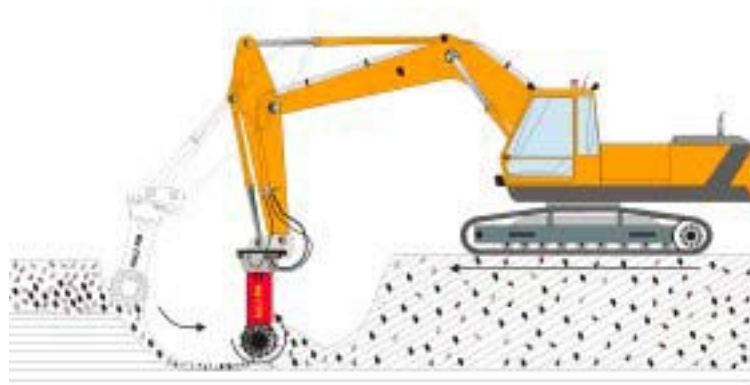
Picture 2. Mixing in layers by ALLU PM Power Mix.
